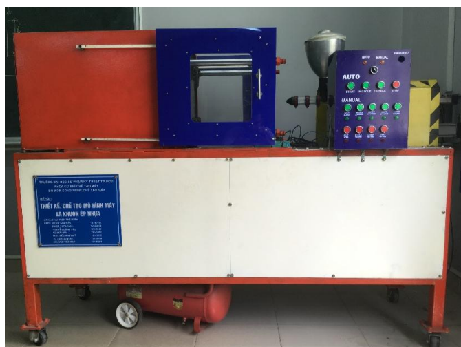
Figure 10.1: Prototype of an injection-molding machine to support teaching in the classroom
